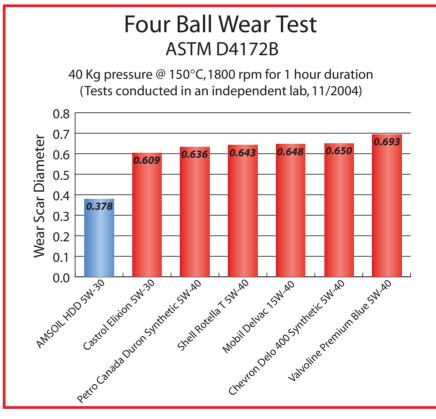
The Four Ball Wear Test (ASTM D4172B), a test designed to measure the effectiveness of anti-wear additive systems, shows AMSOIL Series 3000 Synthetic 5W-30 Heavy Duty Diesel Oil produces a smaller wear scar than competing 5W-40 and 5W-30 oils.
